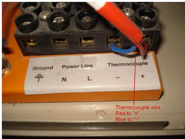
**Fig. 23 : Wire terminals and thermocouple wire**
