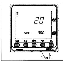
9. With the ⊠ keys, set, for example, 300 °C as temperature of operating.
