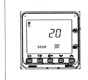
1. PV info-line displays 20°C as a present temperature in the chamber.
