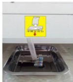
machine condensate water exit
