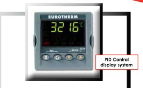
Controller – A digital microprocessor based PID temperature controller controls the temperature within the range ambient +300°C to +1200°C.
