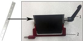
The knife holder is designed for conventional disposable blades from all current manufacturers. It is available in two models: one for narrow-band blades and one for broad-band blades. The knife holder has a lateral movement, so that the entire width of the blade can be used.
