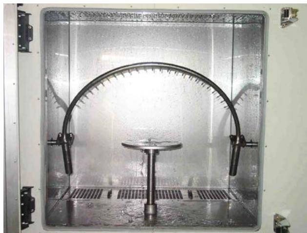
Picture 2: Swing Tube Test IPX3/IPX4
