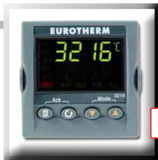
PID Control display system
