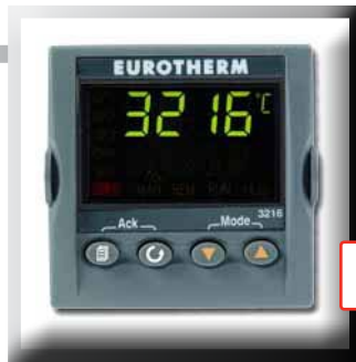
PID Control display system
