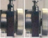
tighten. If the locking pin is hard to lift, you can tighten the handwheel ,the pin will easy to lift.
