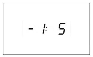
fig. 26 — **Set** parameters. Hold down the **Start/Stop** button to access the parameters. Parameter -1 sets to the dose dispensed by peristaltic pump **P1**. Use the **Selection** buttons to modify the parameter. Use the **Functions** button to move to another parameter. Confirm changes using the **Start/Stop** button.
