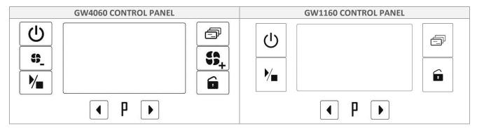
fig. 7 – Control panel. The display and indicator LEDs are in the middle and the control buttons at the sides and bottom.
