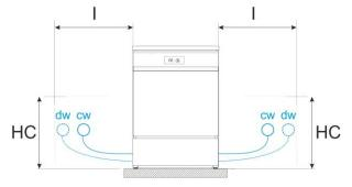
fig. 49 – Diagram. The water supply connections may be on the right or left of the appliance, always considering the maximum distance
