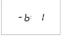
fig. 30 - SET appliance parameters; parameter -b is used to enable and disable overwriting of the internal data memory.
