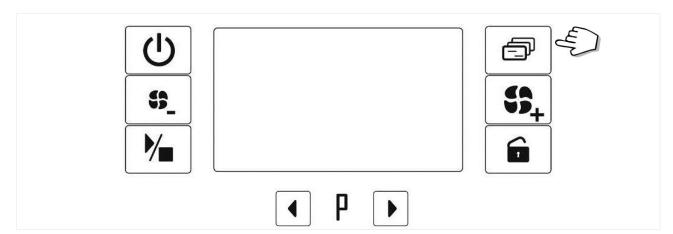
fig. 10 – **Functions** button. With the cycle in progress or cycle selected, pressing the **Functions** button the screen displays the parameters of the washing cycle: A0 value, Temperature and Time Remaining.
