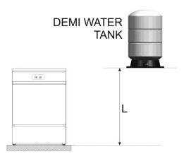
fig. 50 – Unpressurised tank, height above appliance installation surface.
