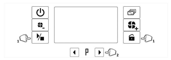
fig. 19 – Demi water disabling buttons. To access the function: hold down the **Functions + Door opening** buttons together. To select demi water disabling: **Selection** buttons
