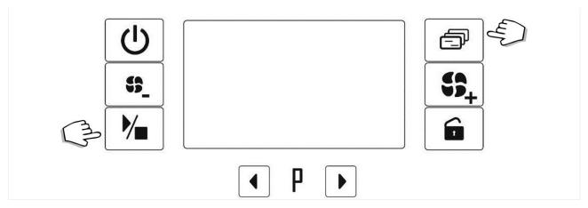
fig. 21 – RESET cycle selection buttons: hold down the **Start/Stop + Functions** buttons together
