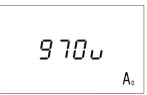
fig. 8 – The AO value is displayed split into thousands (t) and units (u)
