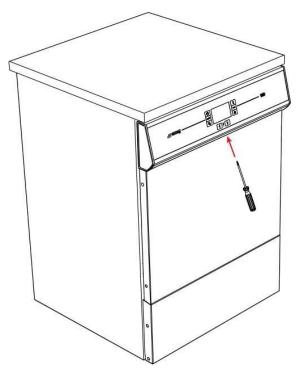
fig.~6-4060 series. Diagram showing how to release the lock by hand in any emergency.
