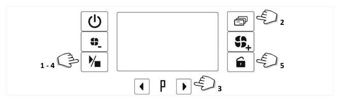
fig. 25 – Steps for display and modification of the **Set** and **Cloc** parameters: **Access the parameter**: by pressing the **Start/Stop** button **Quit the parameter**: by pressing the **Door opening** button.
