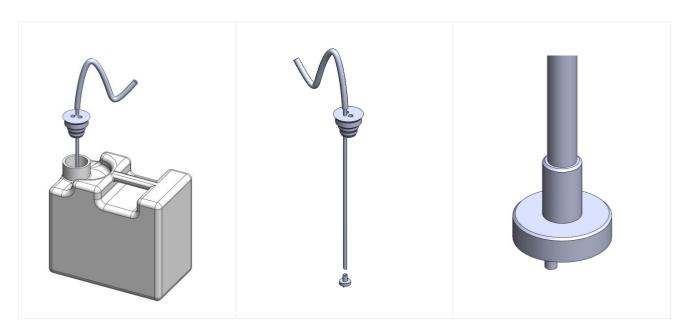
fig. 34 – Detergent intake **STANDARD version**. Fitting the detergent intake pipe to the can. Fit the rubber cap over the top of the can for a perfect, secure connection. The pipe is supplied complete with intake filter.
