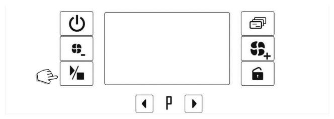
fig. 17 – Interrupting a Program: hold down the  ${\it Start/Stop}$  button
