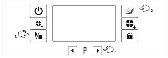
fig. 11 – Standard procedure for **starting a cycle.** 1 **Select the program** using the **Selection buttons.** 2 **Check the** program parameters: **Functions button.** 3 **Start the program**: hold down the **Start/Stop button**.
