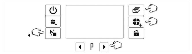
fig. 24 – **Functions** button: hold down to access the Setup mode.
