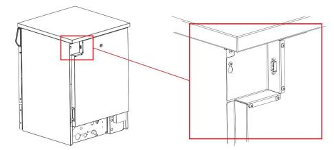
fig. 46 – Rear of appliance, RS-232 port position.
