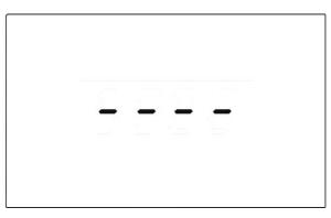
fig. 16 – End of cycle, display screen. The word End indicates that the washing process has been completed correctly. If automatic opening is enabled: the door is released automatically and the 4 dashes appear on the display.
