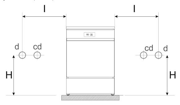
fig. 51 – Diagram. The water drain connections may be on the right or left of the appliance, always considering the maximum distance "I".
