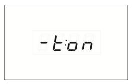
fig. 29 – "Set - t" value can be "--" or "on". In this latter case a test cycle will be activated.
