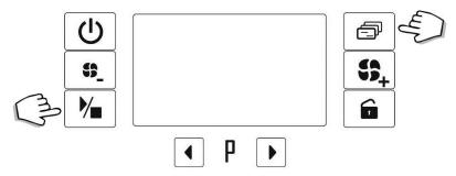
fig. 39 - RESET cycle selection buttons ("Start/Stop" + "Functions") buttons
