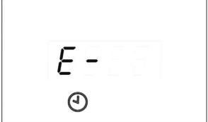
fig. 22 – RESET: during the RESET the display shows "P-". At the end of the RESET cycle, "E-" appears on the display.
