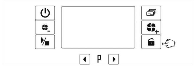
fig. 5 – Selecting automatic door opening
