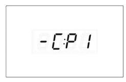
fig. 28 – "Set - C" parameter. The user can fix the use of the powder dispenser (= "dd") or the peristaltic pump (= "P1"). When "dd" is chosen, a possible value saved in "Set - 1" will be ignored by the system.
