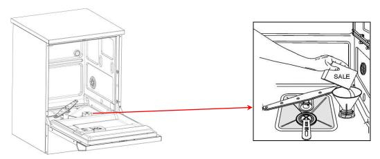
fig. 33 – The salt tank is accessible with the door open; filling the softener tank with regenerating salt.
