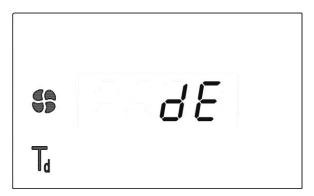
fig. 20 – Display screen: TEMPORARY disabling of demi water; the option can be enabled and disabled using the selection buttons
