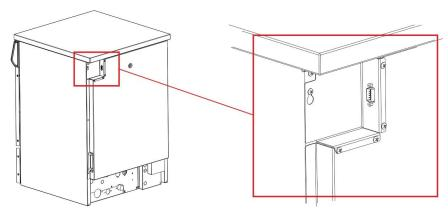
fig. 54 – Position of the RS-232 serial port on the device
