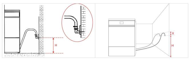
fig. 52 – Drain connection. 65 cm < H < 80cm, X < 20cm. Suffix "C" on the name of the model indicates "equipped with steam condenser", in this case n.ro 2 drain pipes are provided.
