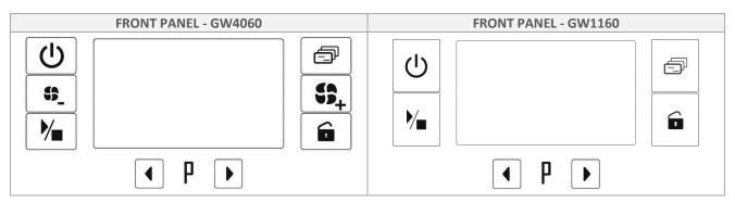
fig. 4 - Front panel; the central part contains the segment display and the appliance control buttons.
