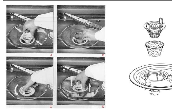
fig. 43 – Draining filters in the chamber; dismantling procedure and detailed view.
