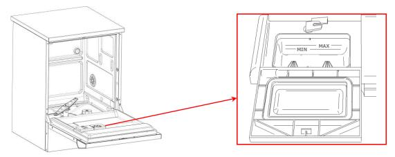
fig. 36 - DD powder detergent dispenser, accessible with door open.
