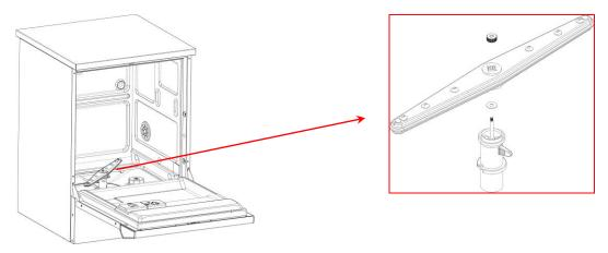
fig. 42 – Appliance bottom spray arm: remove and clean regularly to maintain optimal washing results.
