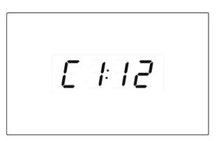
fig. 32 – Cloc parameters. Hold down the Start/Stop button to access the parameters, in this case identified as C1, C2, etc. Parameter C1 sets the current year, C2 the month, etc. Use the Selection buttons to modify the parameter. Use the "Functions" button to move to another parameter. Confirm changes using the Start/Stop button.
