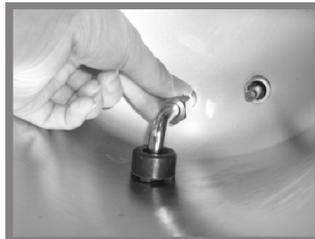
2、 rotate off the filter screw
